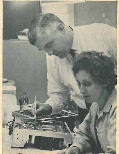
Scott's Chief Kit Engineer, Gaylord Russell, watches while one of 100 novices builds a pre-production sample of a new Stereo Tuner Kit. The unique alignment procedure uses the indicator on the tuner itself, permitting laboratory-accurate results and pinpoint alignment. Even at the hands of a novice, every tuner kit will meet or exceed published specifications.
