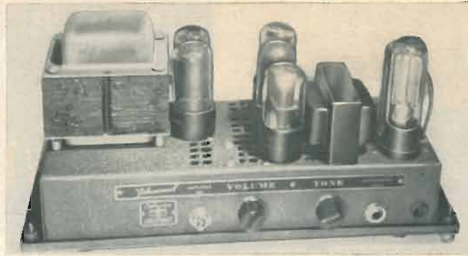
Fig. 4—Fig. 2 amplifier again. Note photocell at right front corner.
