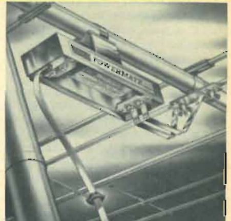
Fig. 5—Best place for booster is at the antenna. Most boosters draw power through signal lead-in.
