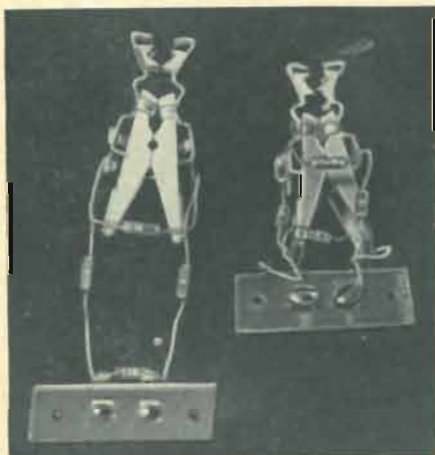
Fig. 3—Carry a few clip-on pads with you to check out suspected overload problems.
