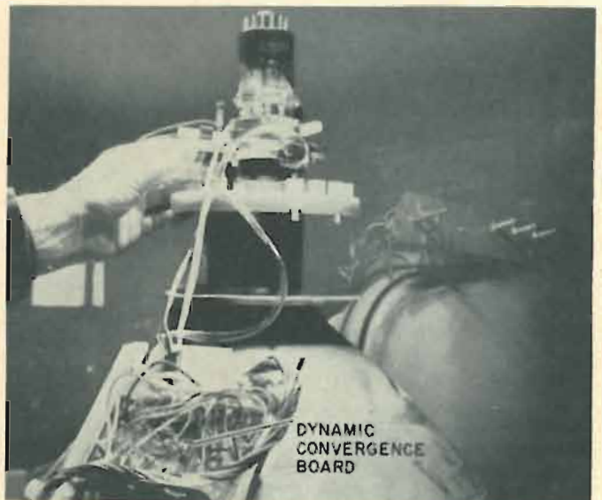
With color tube on bench, start removing yoke and convergence assemblies.
