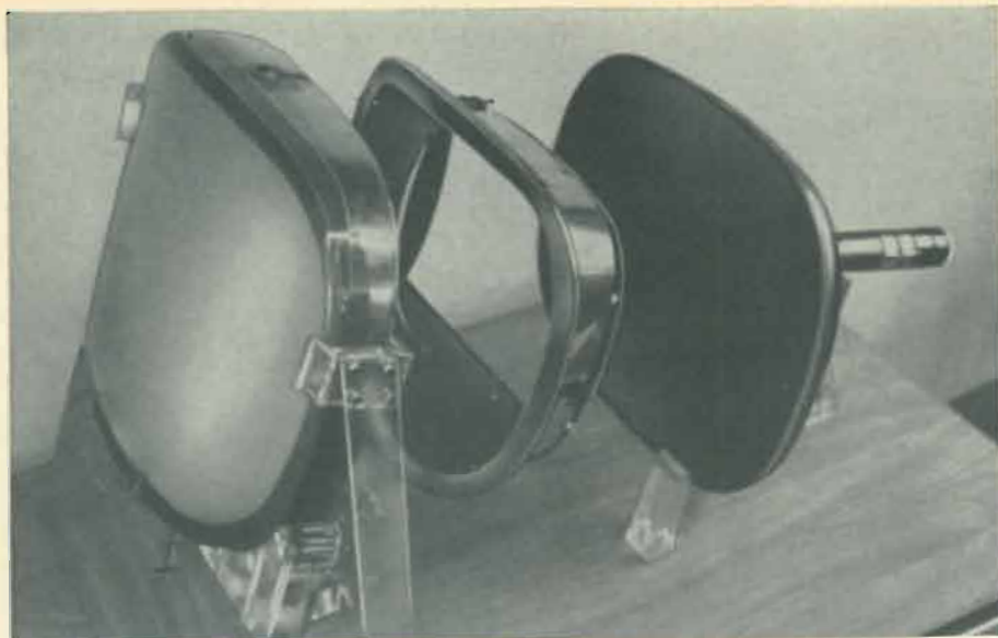
Exploded model of Chromatron. Fine wire grid that deflects electrons onto correct color strip is held by center section, and cannot be seen in photo.
