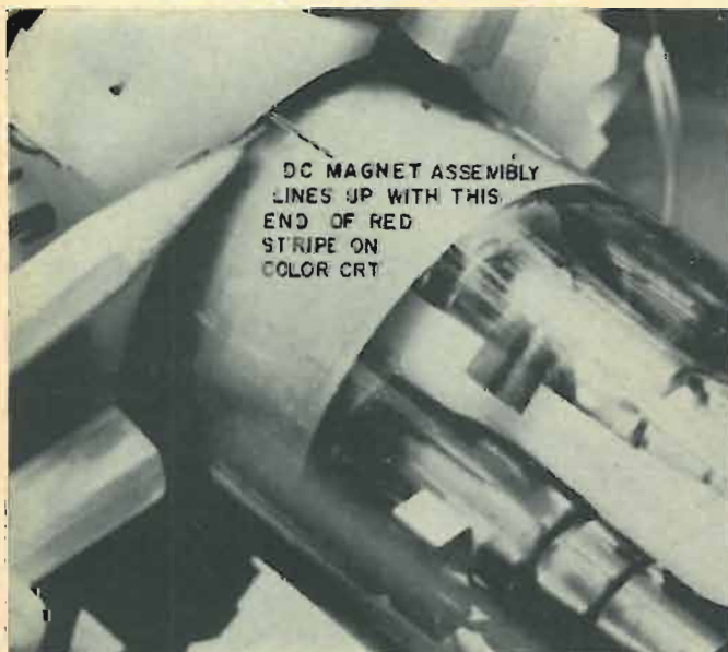
Dc magnet assembly is lined up at this end of red stripe on color CRT
